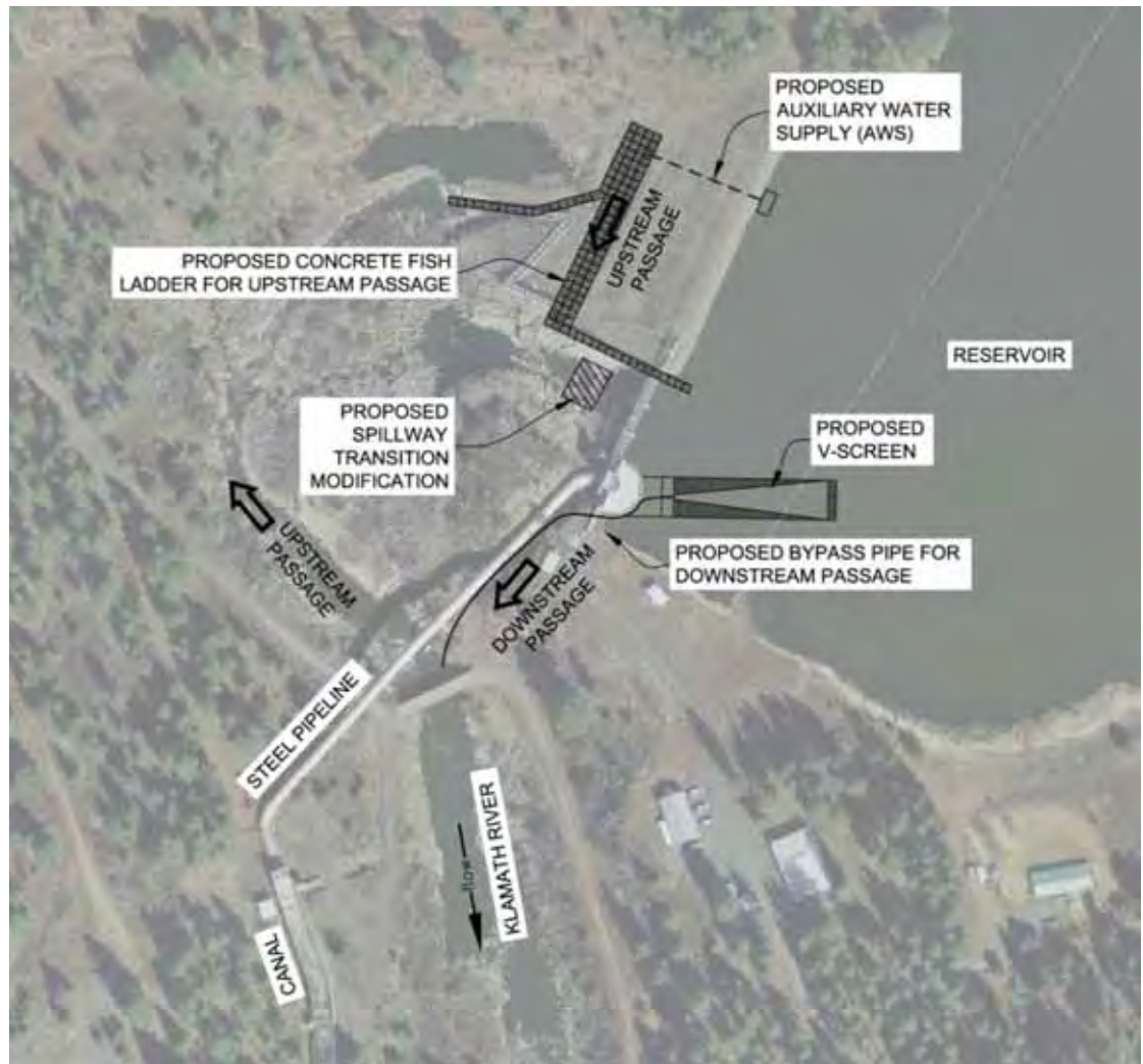
Figure 2-23. Conceptual Layout of J.C. Boyle Fish Passage Facilities
