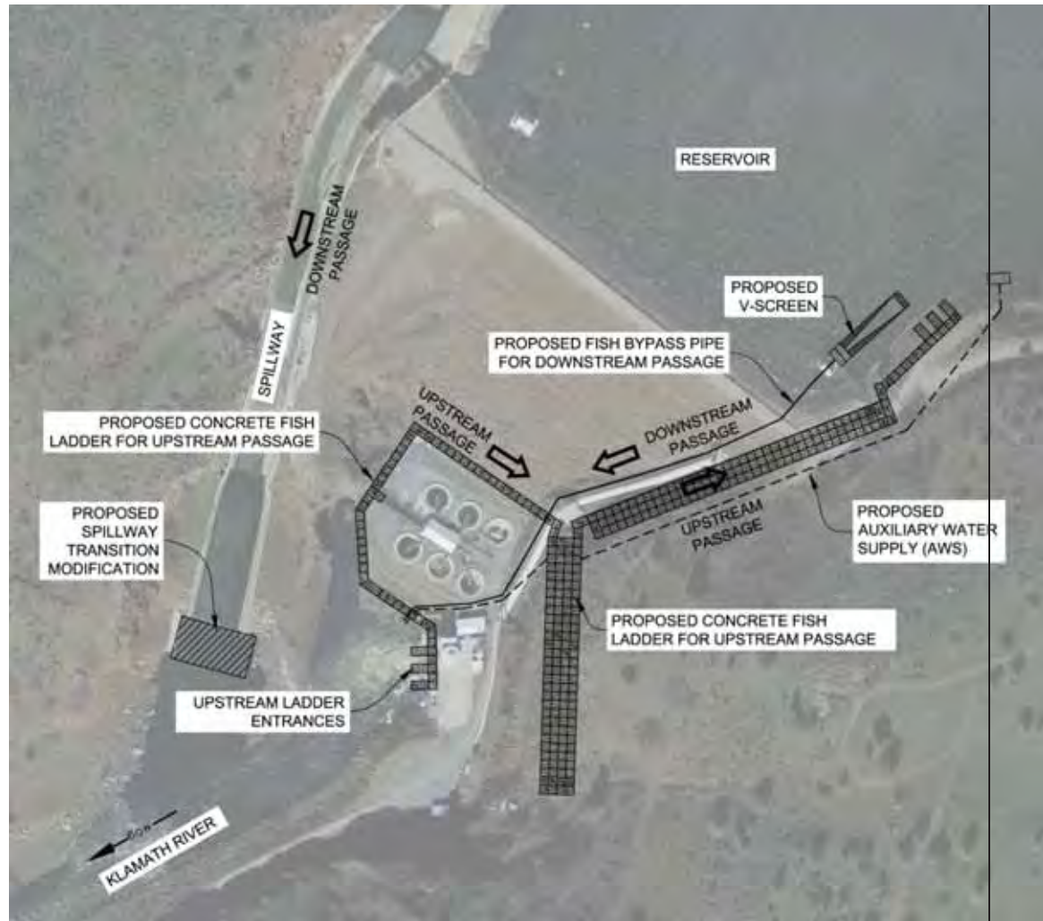
Figure 2-28. Conceptual fish passage facilities layout for Iron Gate Dam showing fish ladder, water intake screen, and spillway transition modifications
