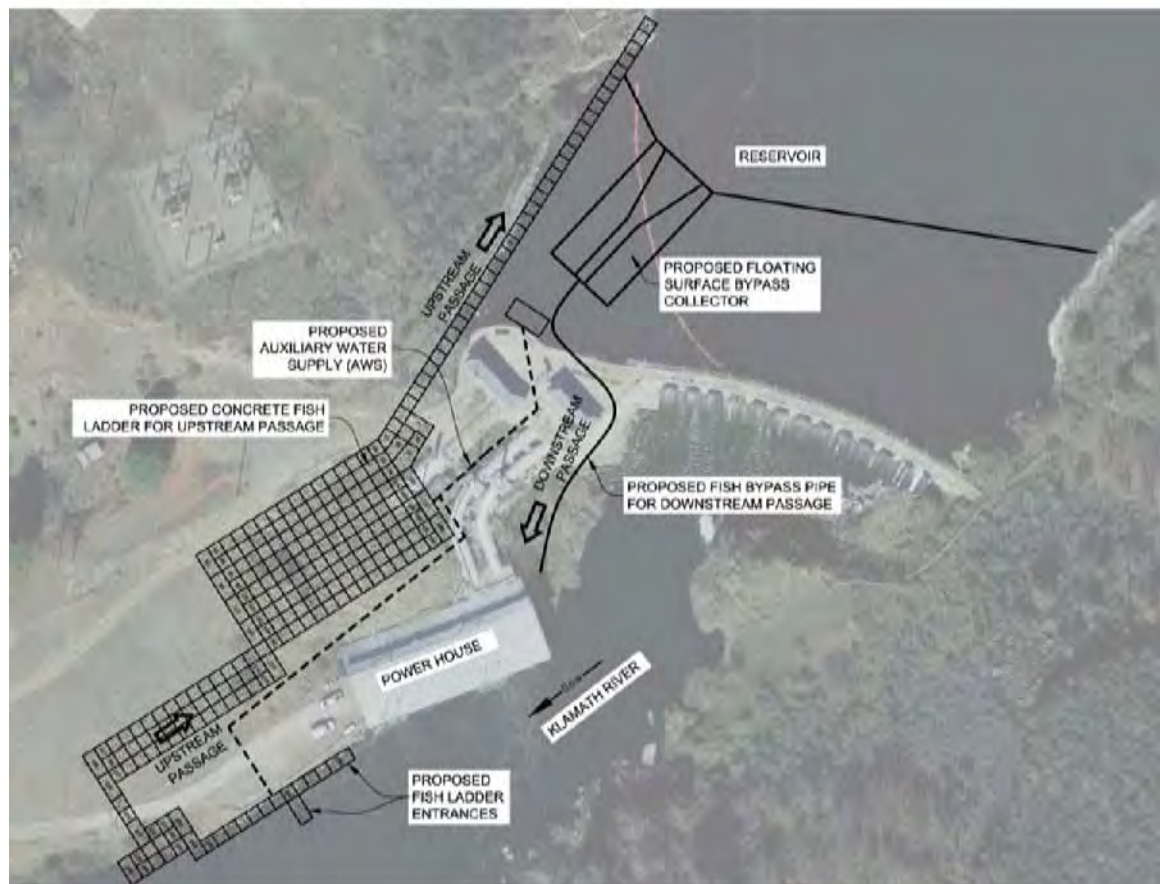
Figure 5-20. Copco 1 Fish Ladder Configuration and Floating Surface Bypass Collector
