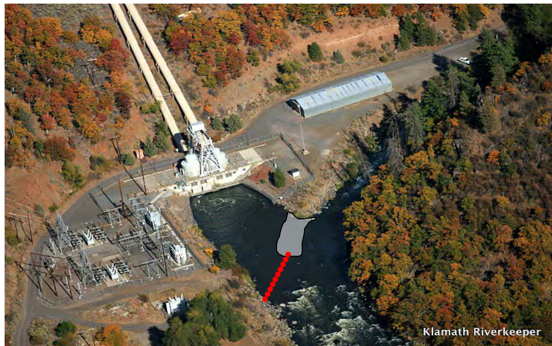
Figure 5-19. Modifications at the Tailrace of J.C. Boyle Power Generation Plant Would Extend the Bank and Install a Tailrace Barrier Screen (red dots) (photo from Klamath Riverkeeper)
