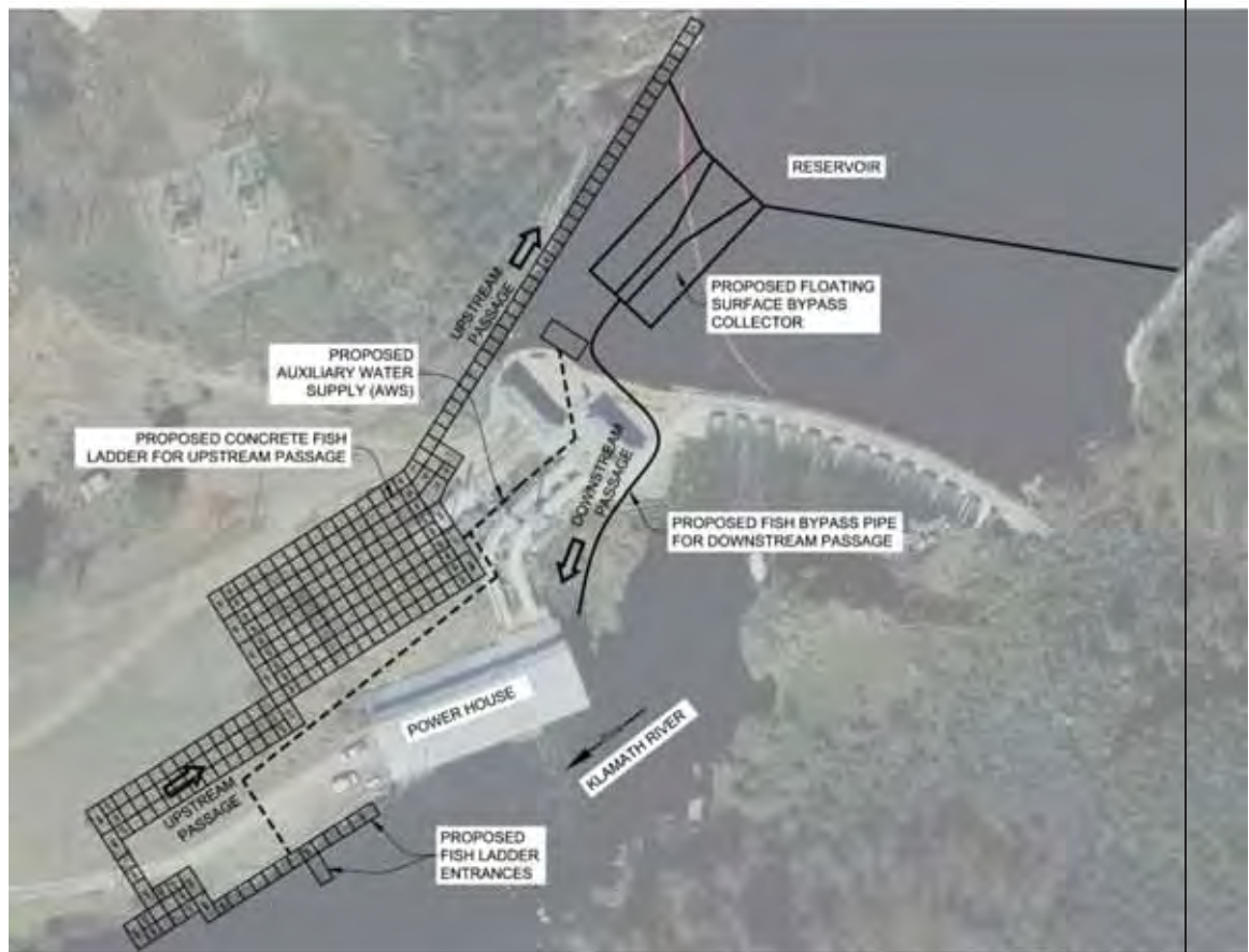
Figure 2-24. Copco 1 Fish Ladder Configuration and Floating Surface Bypass Collector
