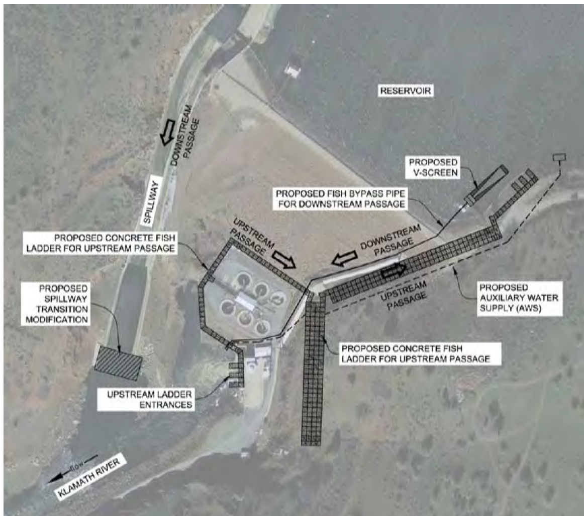
Figure 5-25. Conceptual Fish Passage Facilities Layout for Iron Gate Dam showing fish ladder, water intake screen, and spillway transition modifications
